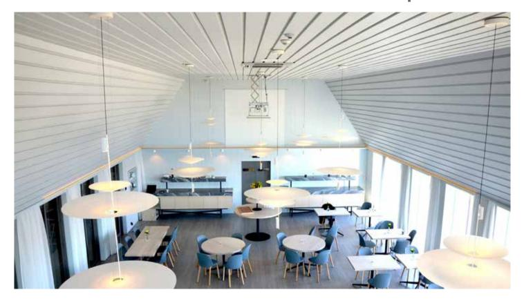
Nordic QVFR White offers invisible protection to B-s1,d0 for indoor walls and ceilings. Nordic QVFR White is a flame retardant paint for protection of wood based substrates.
