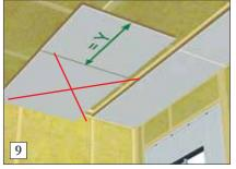
9) This should be measured and marked on the 1st panel in the 2nd row of panels. Cut off the excess section. When cutting with a circular saw, the painted side must be face down.
