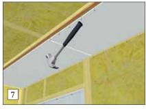
7) The joints must not be glued. Nail spacing is c/c 150 mm. To prevent damage to the panel, a punch should be used when nailing to the final studding. Staples and screws can also be used (see inst.instr. M005-08-04).
