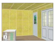
3) Installation usually takes place on longitudinal electrician's laths at intervals of c/c 60 cm. All free panel edges must be supported. When installing narrower ceiling panels, the spacing of the battens must be adjusted to fit the width of the ceiling panels.
