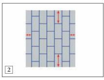
2) The principle of the drawing also shows how to achieve the best layout solution on the ceiling and how the panels need to be adjusted prior to installation. A distance of 7 - 10 mm should be kept between walls and fixed points.
